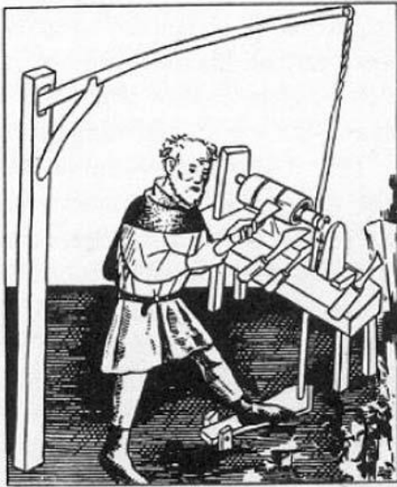
3 A German pole lathe of 1395 (Mendelesches Brüderbuch)
