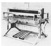
Sturdy, reinforced beater, beveled shuttle race, locking rods to immobilize the beater when sleying, lift out removable harnesses, spring lock hooks, large eye heddle, removable board for pinning up your patterns, one yard sectional warp beam.
