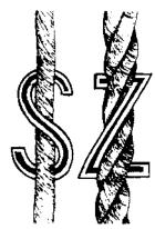
FIGURE 2. S twist and Z twist
