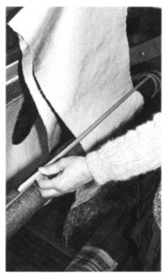
4. Removing cloth from student loom; note tension bar which attached cloth to front beam
