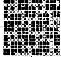
coarse, as it is difficult to insert as many face picks per inch in a filling back cloth as in a cloth without back filling. The result of the more open filling set is that each square of the weave represents a space which in the cloth itself is longer than it is wide. The chief defect of such a texture is that the warp colors are more prominent
