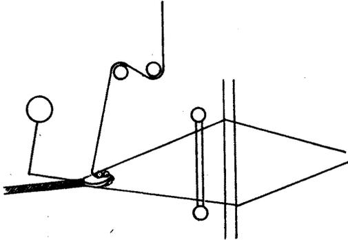
FIG. 16. SHOWING POSITION OF LOOPER AT THE THIRD PICK
