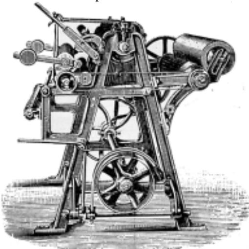
FIG. 3. A SINGLE RAISING MACHINE FOR PIECE GOODS
