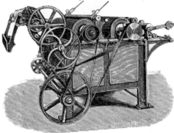
FIG. 2 A DOUBLE RAISING MACHINE WHICH IS ADAPTED FOR PIECE GOODS
