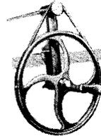
**Leclerc bobbin winder.** A tapered shaft winder built to accommodate **Leclerc** bobbins. Will clamp to a table top and is belt driven.
