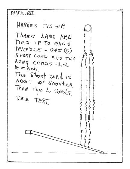
Sem plate detail from aking heddle frames and the heddles. When the new heddles and frames are ready they may be hung permanently in the loom, as with the long and standard eyes, they are suited to all types of weaving. The loom may also be warped up as usual. The only other changes in the loom will be in the tie-up and in the placing of the arm for the support of the shed stick. See diagram.
