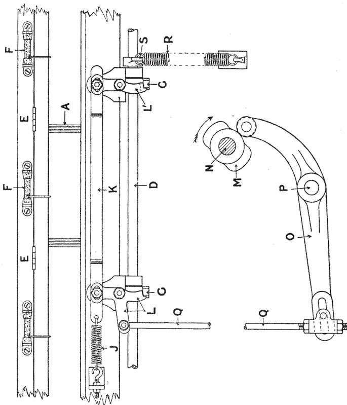
vertical plane, using rod Q as a centre. Should the shuttle fail to clear the shed in due time, pressure between the warp, shuttle and reed A causes the latter to swing back at the bottom and so tilt the extremities of the tongues G
