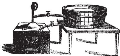
Upon a small scale, the common clay furnaces made in Philadelphia, answer very well to heat water in a copper basin placed upon them.
