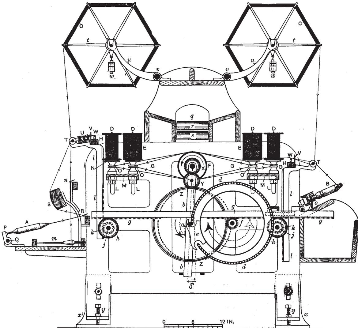
Fig. 5(a).—COP OR BOBBIN WINDING MACHINE (End Elevation).
