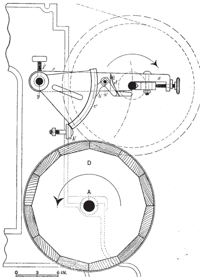
Fig. 58.—BEAM-RETAINING DEVICE.
