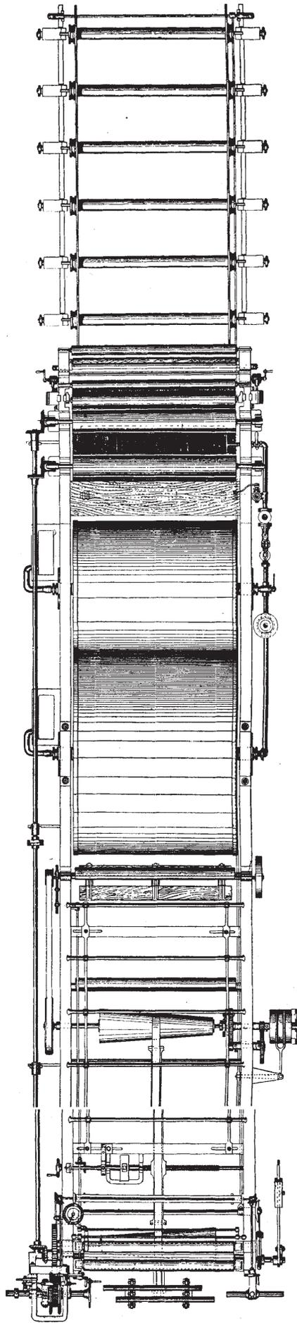
Fig. 68(b).—SLASHER OR TAPE (Cylinder-Drying) SIZING MACHINE (Plan).
