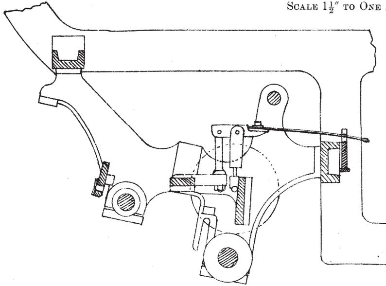
ARRANGEMENT OF LEVER AND WEIGHT FOR PRESSING
