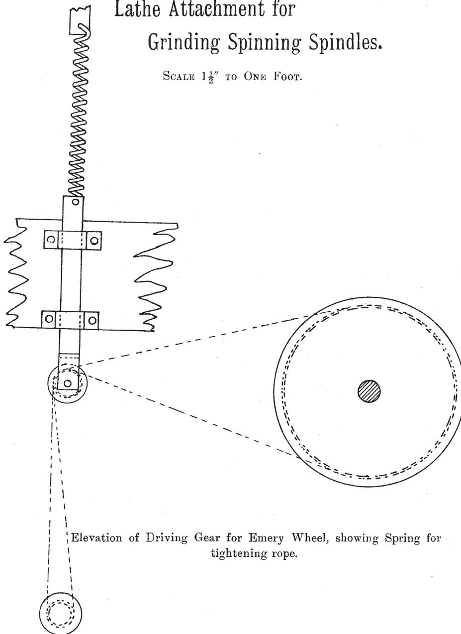
Elevation of Driving Gear for Emery Wheel, showing Spring for tightening rope.
