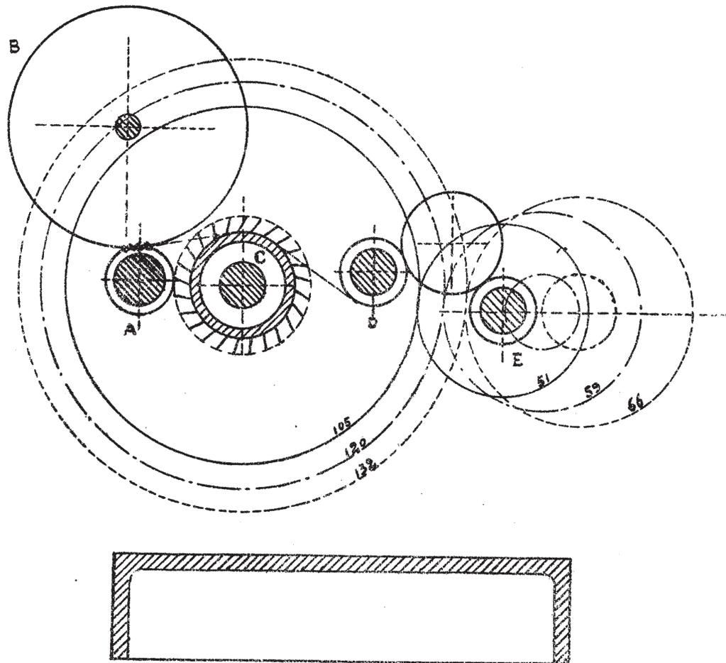
NOTE — The surface speed of the Rotary Gill at the point of the pin is almost equal to the surface speed of the Retaining Roller.
