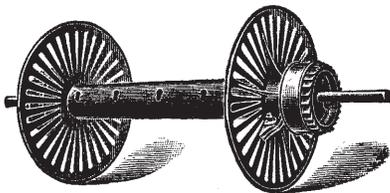
Loom Beams and Flanges.
