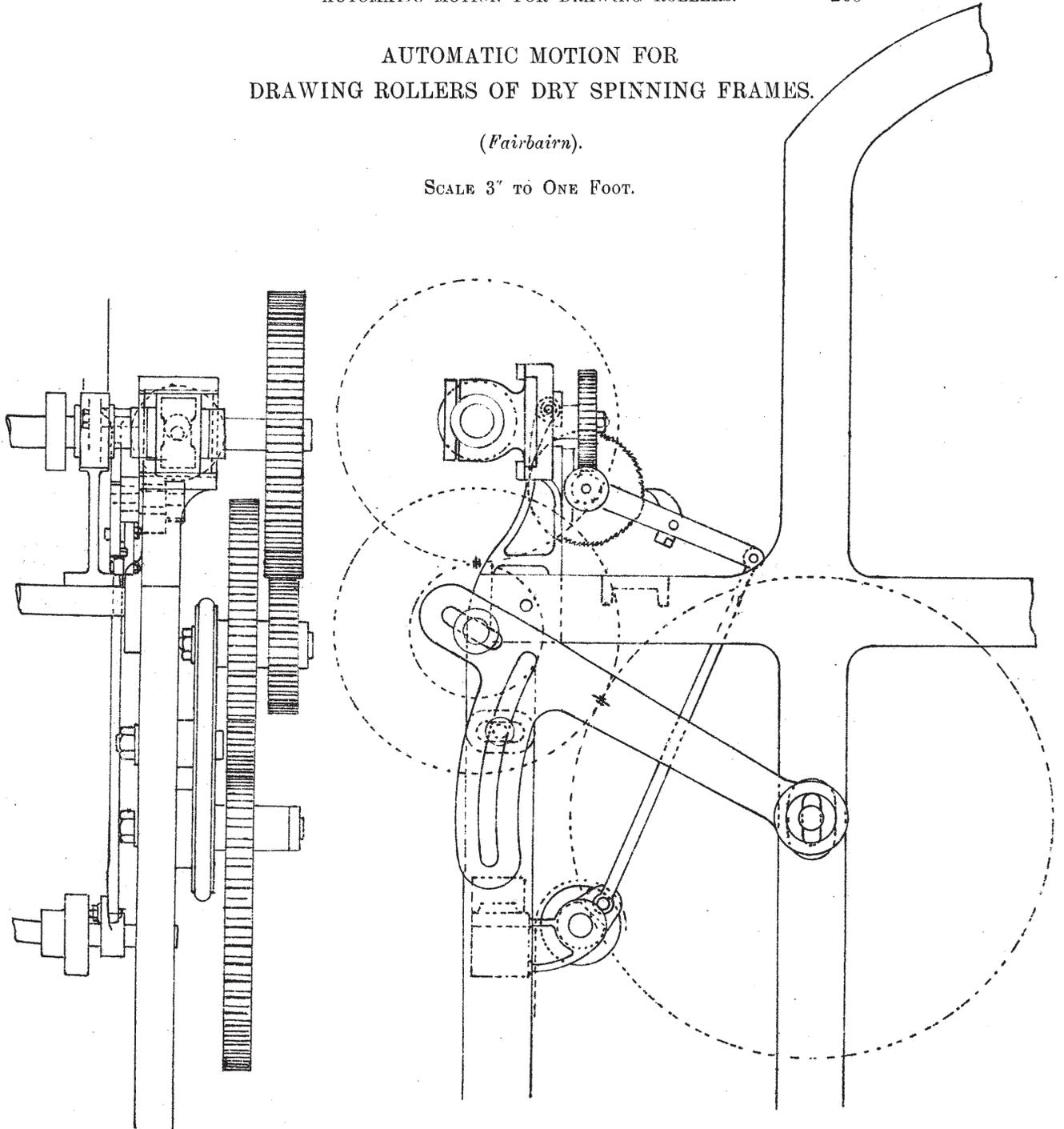
NOTE.—The movement of drawing roller end ways is  $\frac{1}{4}$ " in each direction.
