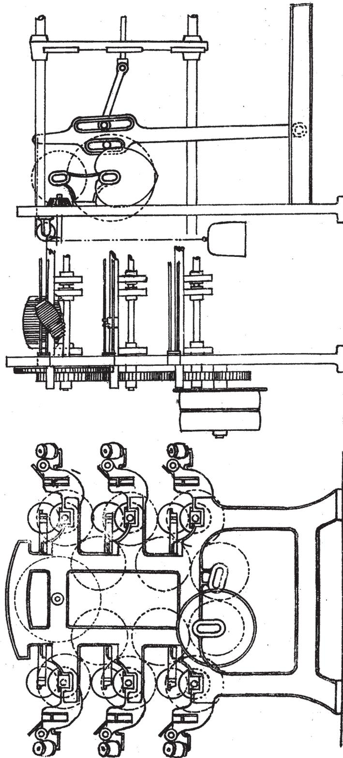
Pulleys 14" diameter. Pulleys Pinion 48 teeth. Pinion on end of Bobbin Drum Shaft 48 teeth.
