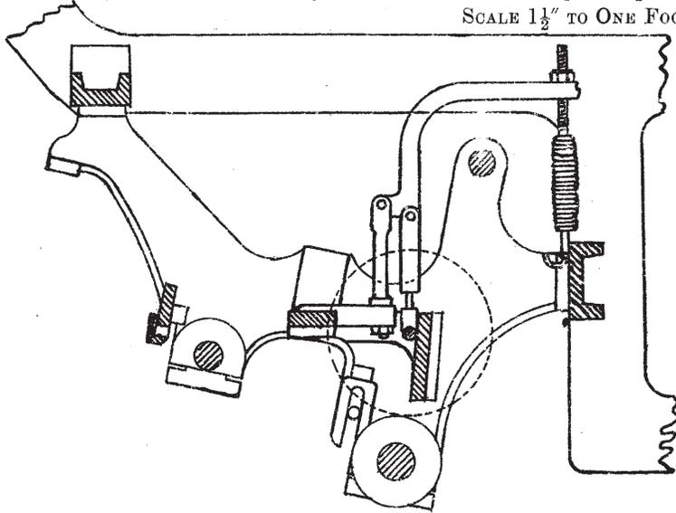
For pressure on pressing roller. Proportion of levers—
