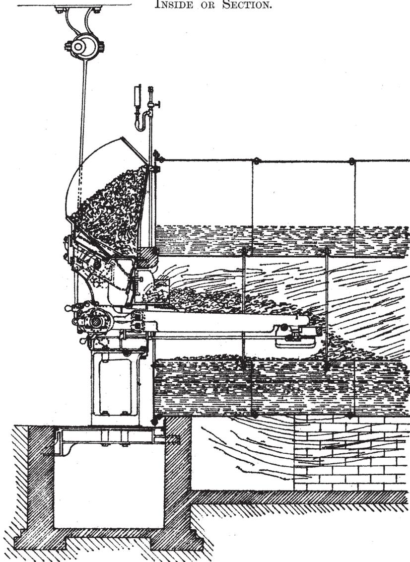
The boilers should be cleaned internally, if the water is of a fair quality, three times a year, and the flues once a year, and the brickwork examined carefully after the annual cleaning is done. The economiser should be "blown through" once a day, and the "soot chamber" and side flues cleaned out three times a year. If the water is of a fair quality, the pipes will not require to be cleaned internally more than once in ten years.
