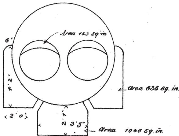
The centre flue is about three feet wide and two feet deep, and the side flues about two feet wide at the bottom, and at the closing-in (which is about three-fourths of a circle) about nine inches wide.
