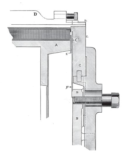
THE ARCH—is so constructed that the flexible is placed close to the cylinder. This flexible is heavier and thicker than any heretofore applied, and overcomes all tendency to buckle. The cut shows a sectional view of the arch, flexible and cut-off plates, and may be described as follows:
