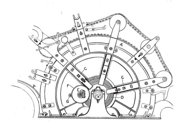
THE FLATS—are 106 in number, 39 working at one time. They are 13/8 inches wide and, clothed to their full length, 15-16 of an inch on face of wire. They are tested and corrected to a 1-1000 part of an inch, both as regards the bevel and the perfect straightness of the wire surface its entire length.
