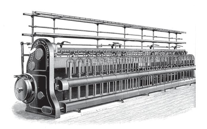
or increase of number of parts over the compound formerly employed. Cut spur gearing is used exclusively in our new compound, and also in the train leading from that to the bobbin shafts, ensuring steady and quiet running. The radial link is made with much enlarged bearings, and ample provision has been made for thorough lubrication of all the parts, which also are very accessible to inspection and easy of repair.
