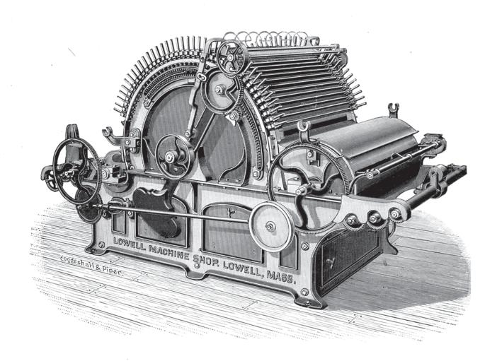
SPACES — The cotton in passing from the leader to the cylinder goes under a steel back plate, which fills up the space, is circular in shape, and adjustable in all directions, and can easily be removed and replaced without disturbing the adjustment. The space between the last top and doffer is closed up by a similar steel plate and equally adjustable.
