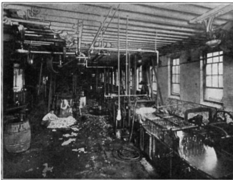
FIG. 70.—Wool Scouring Machinery.
