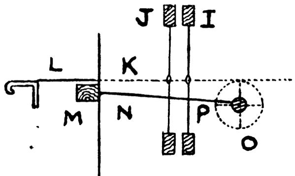
Fig. 30. Late Timing with Crank at Front Centre.
