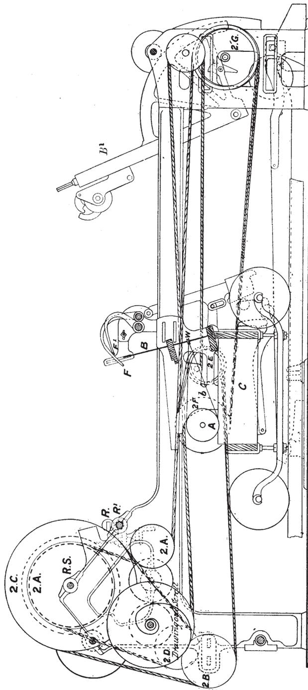
FIG. 83. Self Actor. End Elevation.
