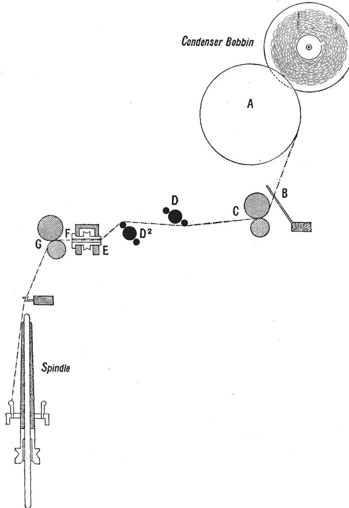
FIG. 90. Sectional Drawing showing the passage of the thread in the Continuous Woollen Frame (Sykes).
