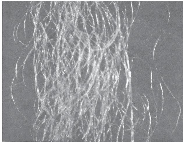
FIG. 91. Sliver from Condenser Bobbin.
