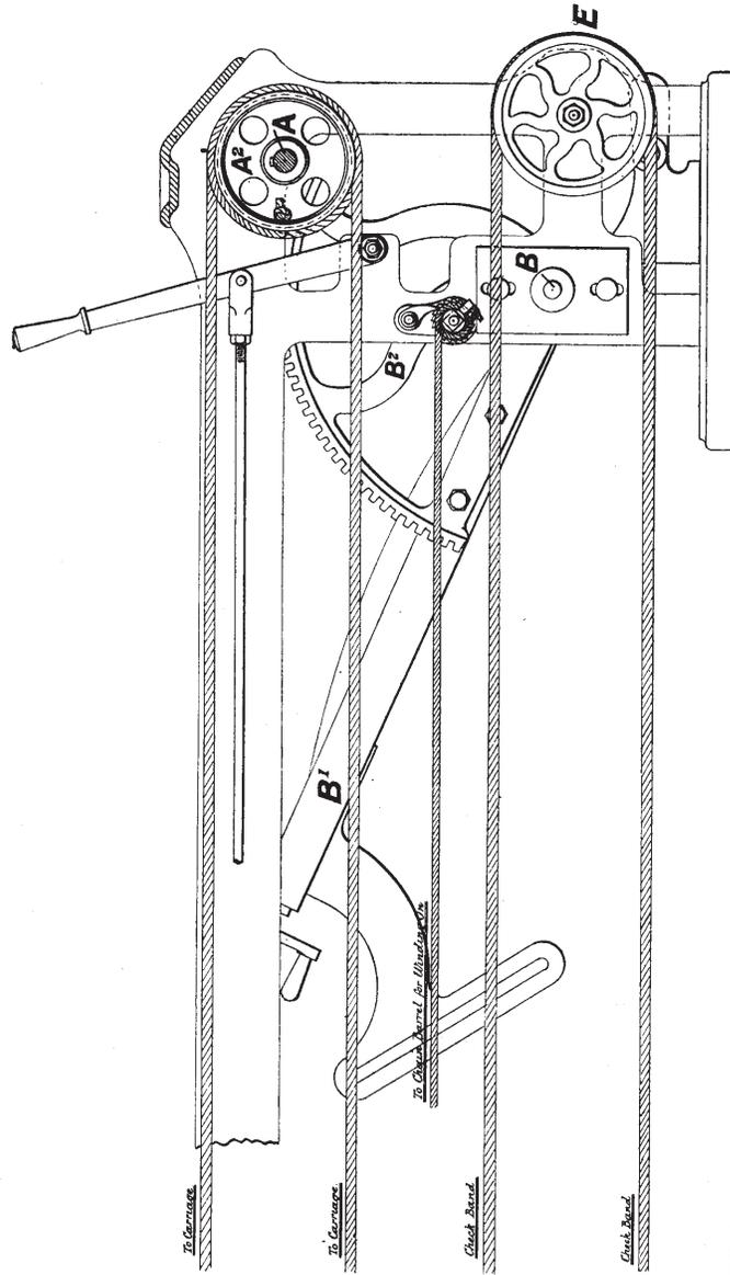
FIG. 88. Section of Self-Actor—Quadrant Motion.
