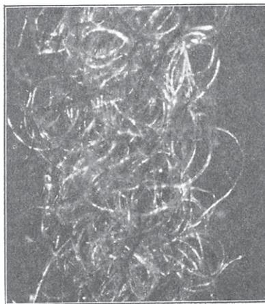
FIG. 78. Condensed Sliver, Pulled Waste.
