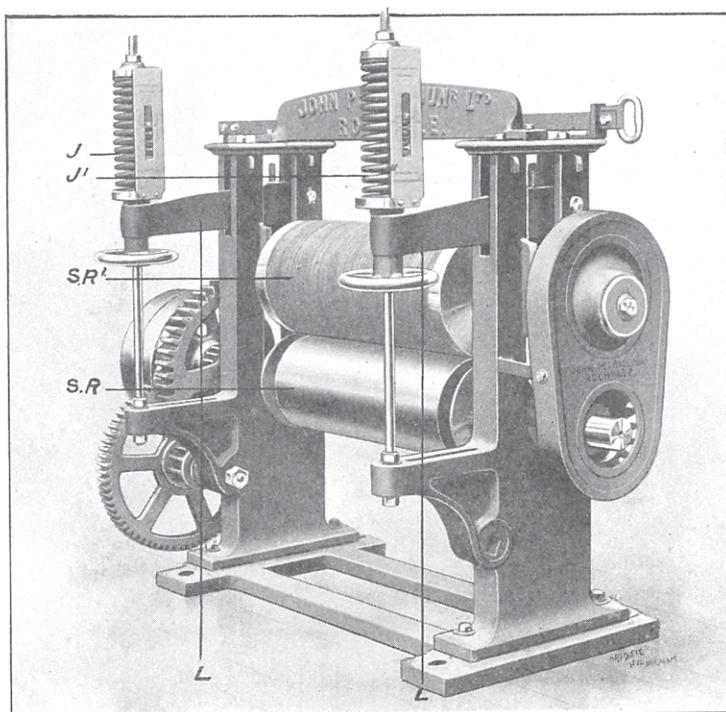
FIG. 21. Arrangement of Squeezing Rollers as applied to Petrie's Wool Scourer.
