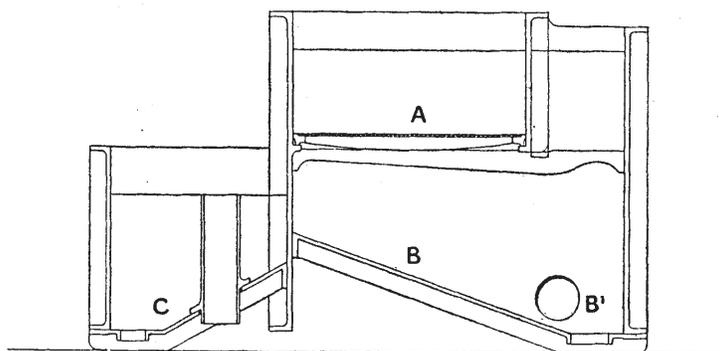
FIG. 17. Vertical Cross Section of McNaught's Wool Scouring Machine.
