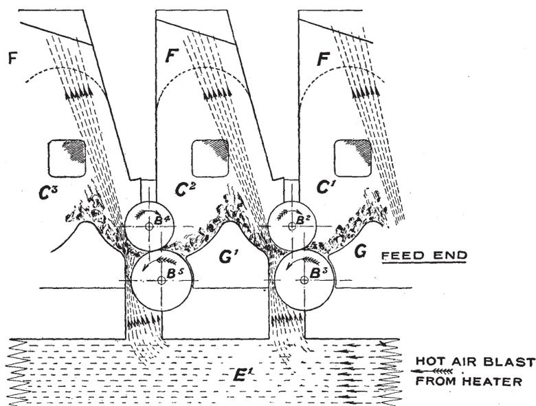
FIG. 26a. McNaught's Continuous Wool Drying Machine (Compartment Method), showing direction of currents of heated air and their action on the wool.
