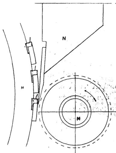
FIG. 34a. Section of Sykes' Burring Machine, showing relation of the Cylinder Blades to the Comb.
