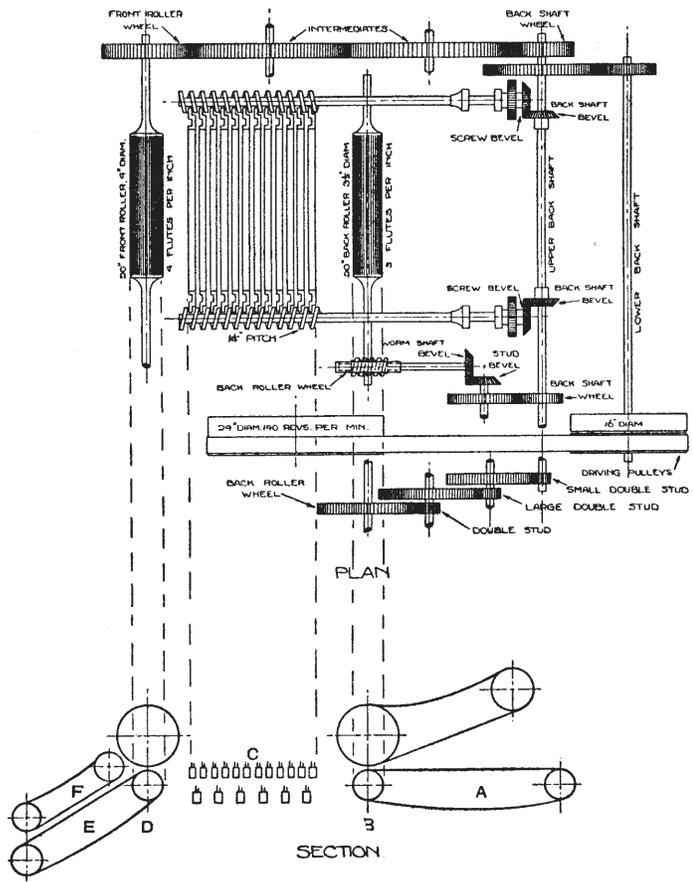
Fig. 87.—Plan and Section of "Sheeter" Preparing Box
