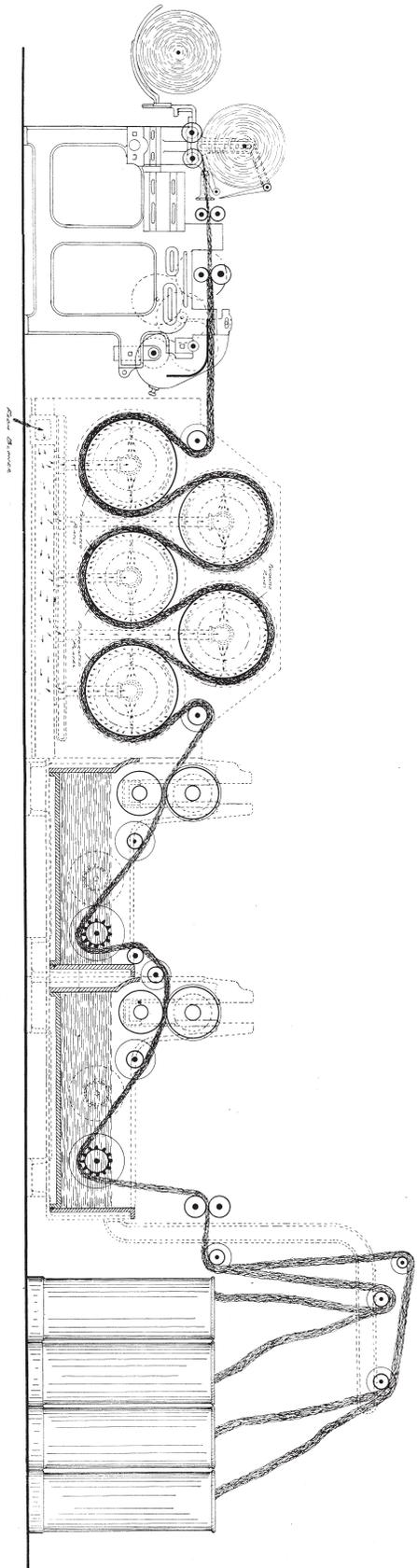
Fig. 93.—Front Elevation of Backwash and Gill (Howarth and Musgrave's Patent)
