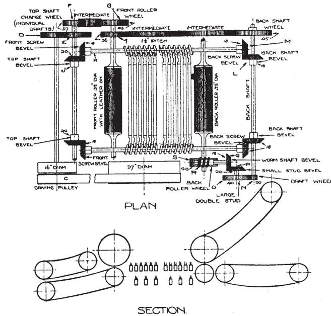
**Fig. 89.**—Plan and Section of the “Clough” Preparer-Box
