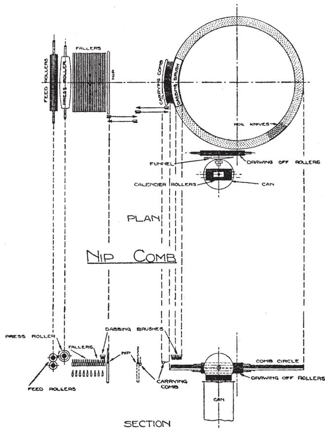
Fig. 100.—Plan and Section of Nip Comb
