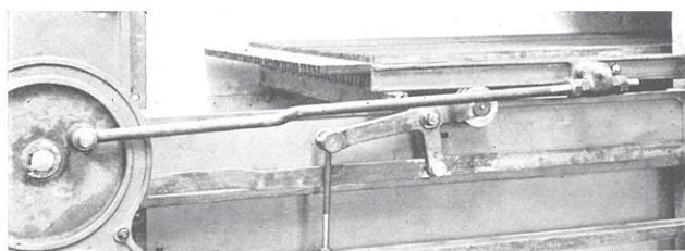
Fig. 71—Showing Action of Drying Machine Shelves
