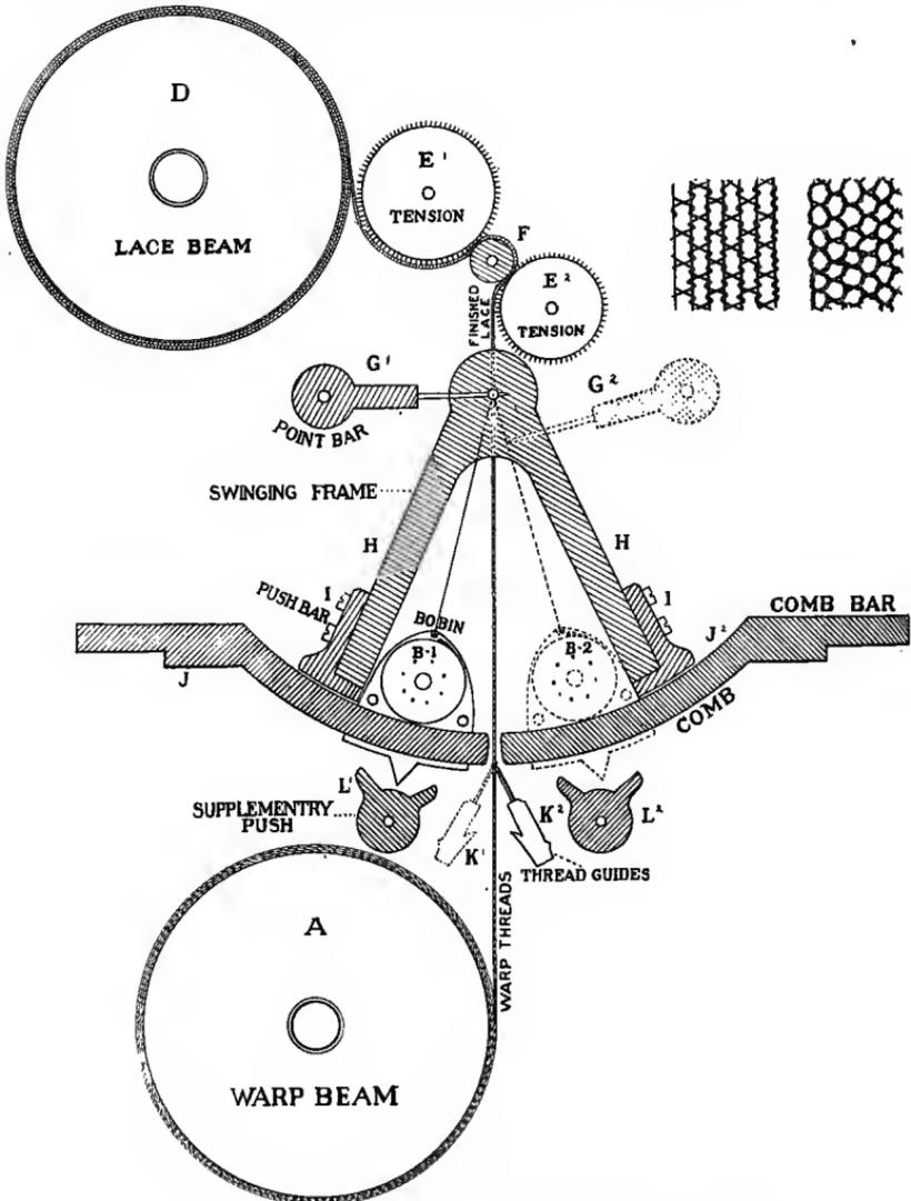
FIG. 6. SECTION OF LACE MACHINE ONE-THIRD FULL SIZE.
