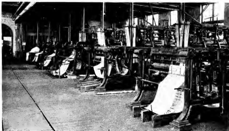
THE average length of lace, thirty yards, is woven in 30 hours. Workmen then unwind the lace from the machine, and pile it in great white heaps.
