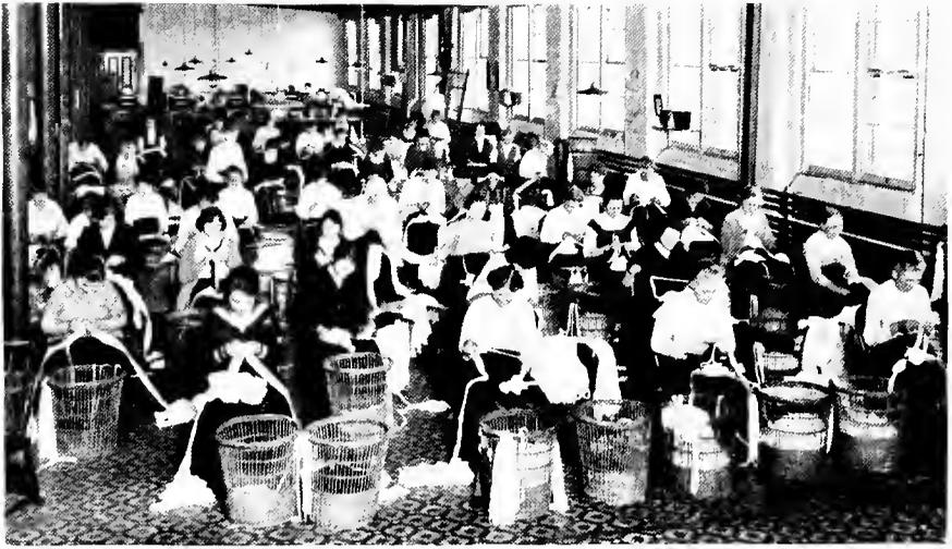
A BLOCK LONG is the finishing room. Here the beautiful web is drawn, and the breadths are separated by pulling the threads between them. The lace is then carefully clipped by hand, and all superfluous threads removed. The next process is to handcut the scallops before the laces are ready to be measured and carded.
