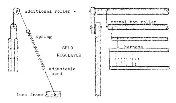
When we do not need the shed-regulator, we use by-pass cords instead of springs. The by-pass cords are of such a length as to keep the shafts in their normal neutral position, that is half way up the reed. The by-pass cords may be also adjustable for very precise control of the shed.
