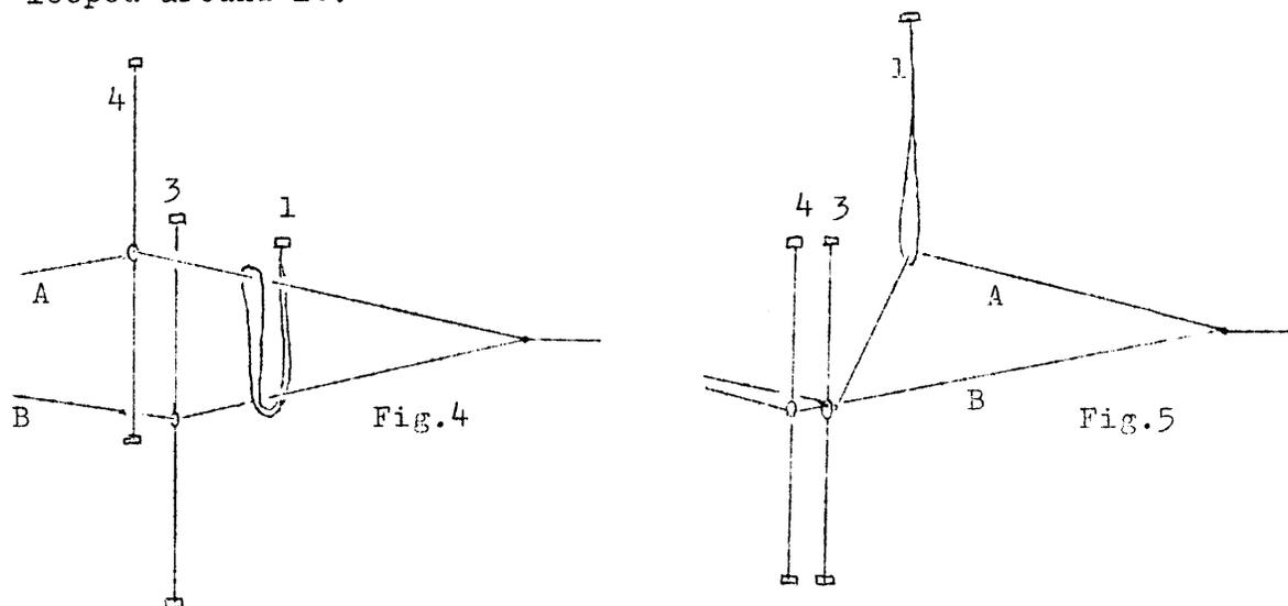
Now we prepare a warp of plain or mercerized cotton No.10/2. We can set it at 16 ends per inch, and use No.8 reed. The threading is done as follows (see fig.6, next page). In each repeat of gauze we take first the end A and pass it through the heddle on frame No 4, and then through a doup on frame No.1. Then we pass the threading hook to the left of the doup (which is already threaded), and
