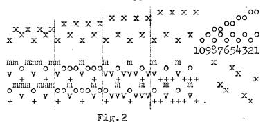
To get four colours we have to make four shots of weft each with a different colour, and each in a different block (fig. 2) in such an order that the ground frames (1 and 2) will be used alternately. Then another four shots on remaining treadles,
