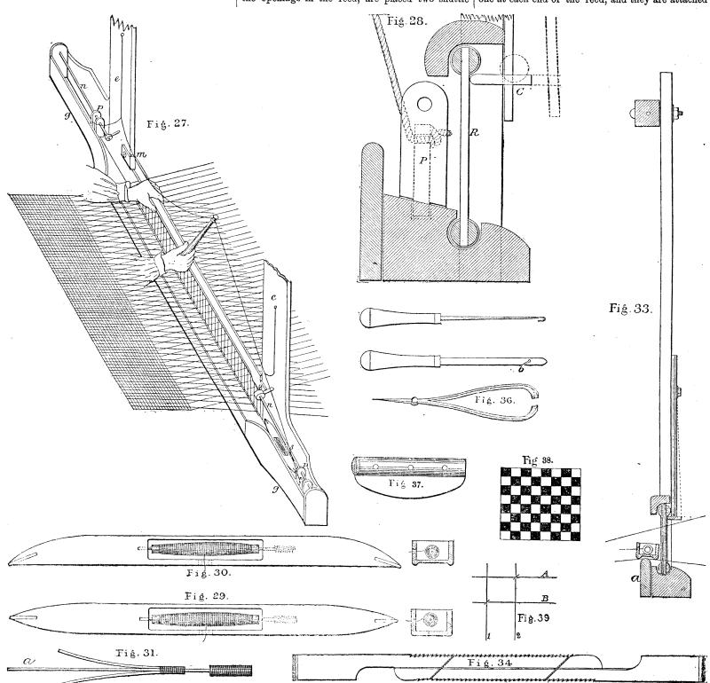
boxes, gg. These boxes have a spindle fitted length-ways over the centre of them, upon which the picker, a kind of hammer, is made to slide. The two pickers are connected together by a slack cord m, to the centre of which the "picking-stick" is attached. Two short ends are connected to the picker cord to keep it suspended and free to work.
