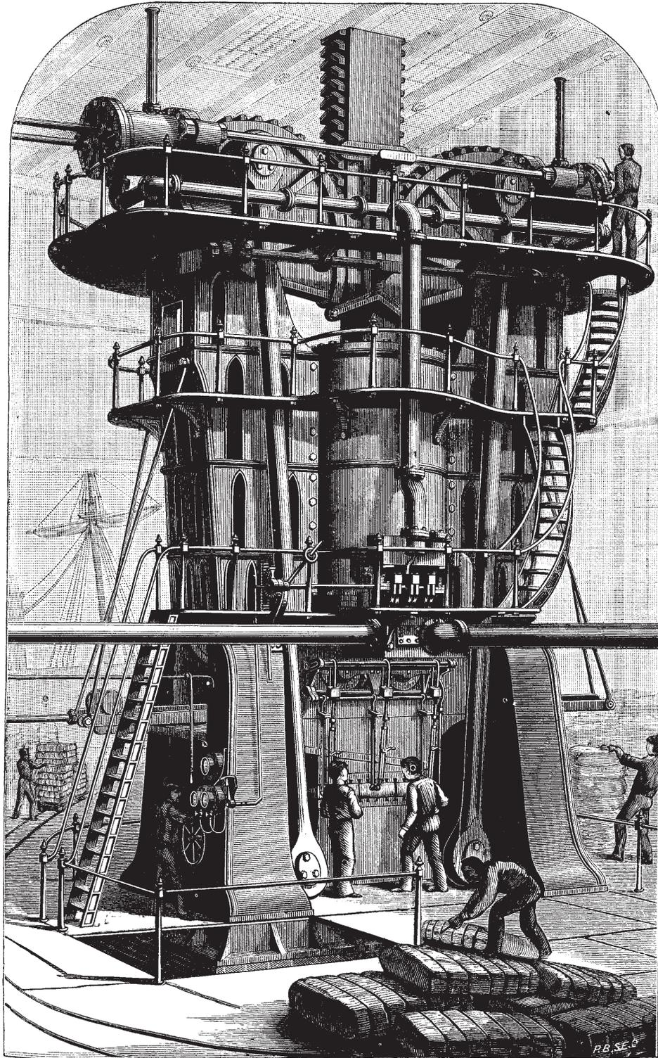
and at others to be several inches within the outer edge of the platens; it must apply the same and consequently an independent strain to each and every band; it must be so simple in its action as to enable any ordinary laborer to use it; and it must be capable of attaining a speed of at least 60 bales per hour. The tie must be self-locking, instantaneous in its action, securing the bands at their ultimate point of tension, and must not impair their tensile strength.
