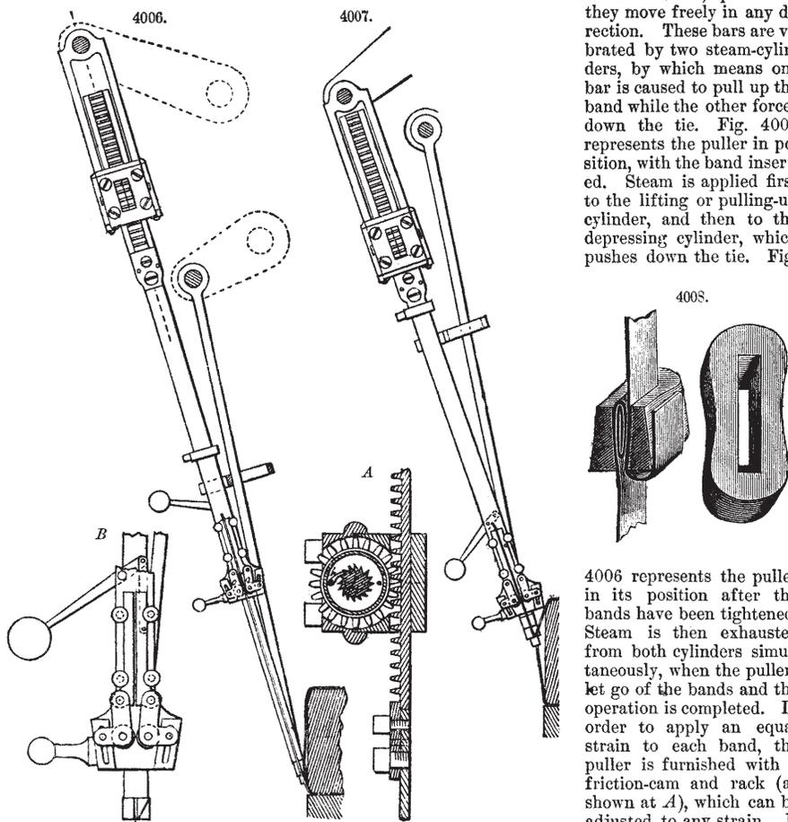
horizontal bars, upon which they move freely in any direction. These bars are vibrated by two steam-cylinders, by which means one bar is caused to pull up the band while the other forces down the tie. Fig. 4007 represents the puller in position, with the band inserted. Steam is applied first to the lifting or pulling-up cylinder, and then to the depressing cylinder, which pushes down the tie. Fig.
