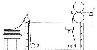
shown in the illustration. There is also a guide through which the cloth passes before entering the squeeze rolls. The opening in this guide should be 4 or 5 in. wide so as to bring the cloth into small compass for squeezing.
