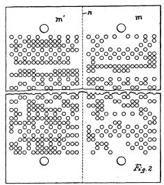
such a duplex head, as used in connection with a regular piano card stamper, clearly showing the two series or sections of keys and punches. Fig. 2 shows a stamped card.
