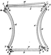
frame is provided respectively with a fixed outwardly extending pivot ear 7 and with a laterally extending pivot aperture 8; the latter extending through a portion of the frame bar which is provided with a slot 9.
