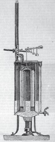
The apparatus is made in three different sizes (a) for single determinations; (b) for three at once; and (c) for six at once. As 300 grammes of material of average moisture usually need about four hours, so in 12 hours a c apparatus can make 18 determinations. The b and c apparatus are intended for steam only; the a apparatus is arranged also for gas or petroleum.-Textil
