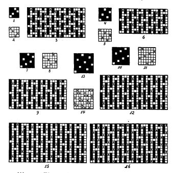
Weave: Fig. 1 shows the 4 harness broken twill: 3 up 1 down (single cloth).
