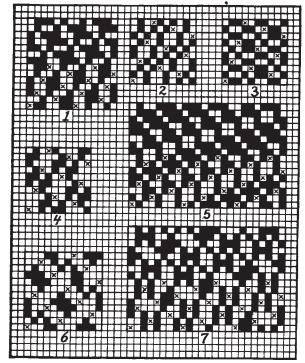
Weave Fig. 3 shows also by  $\times$  type, the foundation for this "Granite-effect"; its basis being the 10 x 10 Satin Weave; showing its construction by  $\times$  type; imparting to the face of the fabric a spotted effect.
