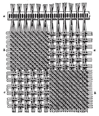
some distance. In the warp these breaks are separated by the reed by leaving one, two, three or more dents empty. The threads requiring for a close working are drawn in one dent. To give a clear explanation of the matter, the accompanying illustration will clearly explain this method of combining the plain weave and imitation gauze for forming figures can also be applied to ornamental or floral designs.
