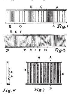
Fig. 1 illustrates a reed in which all the dents run at a right angle to the bars A. The dents of the groups B are at shorter distances a part than those of the group C.
