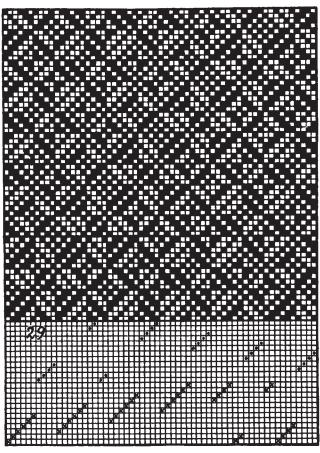
below the weave in *cross* type for one of the twill effects, and in *dot* type for the other twill effect, and will explain how to draw this broken twill systematically on 20 harnesses for practical work on the loom, using 12 harnesses for one effect and 12 harnesses for the other effect of the 12-harness foundation twill, previously referred to.
