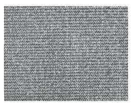
The fabric is composed of white Japan tram, or other kind of nett silk, twisted together either with a white artificial silk thread or a white cotton thread and then knitted to form the fabric into a sock, stocking, undergarment, necktie, etc., after which the fabric is boiled-off in the usual way to remove the gum from the nett silk
