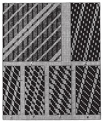
The angle, i. c., the steepness of the present diagonal twill or cord effect will be more acute than those of 70 deg. grading, since in the present instance we use only every fourth warp-thread of the foundation twill, whereas in the construction of the diagonals explained in the January issue, we used every third warp-thread of the foundation twill.
