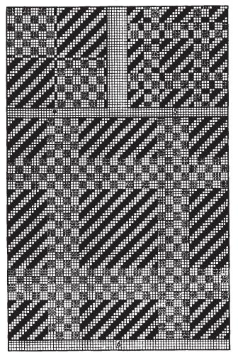
warp-threads and 13 picks interlaced with the 6-harness even sided twill. Complete basket effects are shown by means of dot type, whereas such as had to be modified, in order to produce the clear cut-off on all four sides of the square, are shown by means of cross type. Repeat of weave 38 warp-threads and 38 picks, which by means of a fancy draw, can be reduced to six (or more) harnesses.
