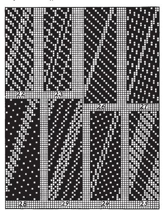
Figs. 11 and 12 show two examples of 70 deg. twills, repeating on 7 by 21, with 21-harness regular twills, respectively for their foundation. We have shown again one repeat warp ways and two repeats filling ways, of the steep twills.
