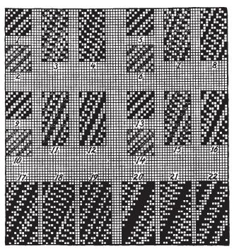
Using pick 7 will give us the same combination, i. e., weave, as pick 6 has produced, in turn resulting in diagonal Fig. 16.
