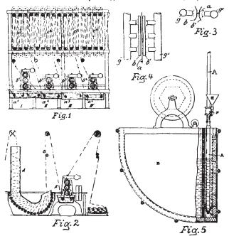
tween each. After this the cloth is piled down in the container d and finally washed off through the pad c.
