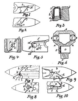
d and passage e. The usual wire curl is replaced by pins j, k, the latter of which prevents the weft from re-entering the groove h after the shuttle has been threaded. One or more drag-pins, such as the pin i, may be placed in the respective thread passages to tension the filling.
