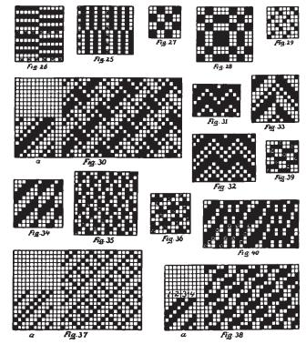
(G) Fancy Twills Obtained by Section Drawing. Weave Fig. 38 explains subject. a is the foundation twill, the  $\frac{2}{1}\frac{2}{3}$  8-harness twill. The same is divided in 4 sets of 2 threads each, viz:
