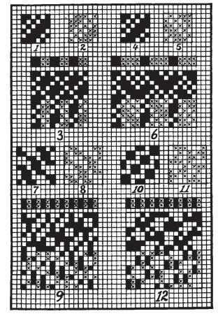
higher—it follows, that in this instance warp-threads 3, 4, 5, 6, 7 and 8 of the crêpe weave (since 9 and 10 = 3 and 4 as above mentioned) form its repeat; hence 6 warp-threads and 6 picks the repeat of crêpe weave Fig. 3.
