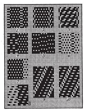
for each of the two cords in the repeat of the weave. If such is desired, use a different color for each section of the warp, using a corresponding or harmonizing color, for the respective pick covering it. Section 1 (warp-threads 1 to 8) of our weave has its binder picks interlace with the 4-harness basket weave, section 2 (warp-threads 9 to 16) interlacing with the plain weave. Repeat of weave: 16 warp-threads and 8 picks.
