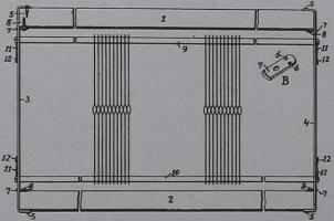
inasmuch as the slotted engagement of said securing braces with the end straps 3 and 4, will readily permit such shrinkage or expansion, without affecting the rigidity of the structure.
