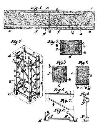
Fig. 1 shows a girder in which the anchor-member a is formed at one end, so as to fit snugly around the main reinforcing bar b, on three sides; and this end terminates in a finger c which lies in prolongation of the side d when the anchor-bar is placed upon the reinforcing bar b and before the concrete is placed.
