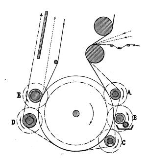
The design or effect desired for the printing, i. e., the coloring of, or the discharging of color from the ends of the protruding fibres, is regulated by means of an engraved roller, and consequently differs from the older process, where a similar result was obtained by means of a brushing process, which however, does not produce the nice smooth even result as the new process does.
