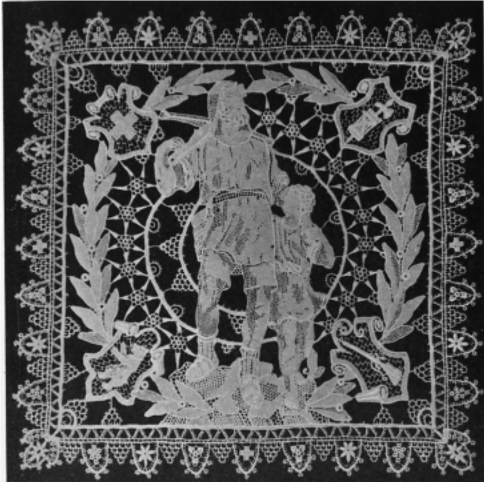
BURNT OUT LACE MADE IN IMITATION OF POINT PLAT DE VENISE BY THE SWISS HAND-EMBROIDERY MACHINE IN 1904 FOR THE ST. GALL RIFLE CLUB.
