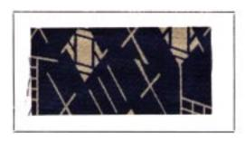
azol B (diazotised and developed with Develsoper ON); it turned out, however, that the shading dyestuffs, used in connection with them underwent so great a change during diazotisation and developing that it was not possible to obtain dyeings of good discharges ability.
