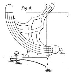
from the number, and from these enough yarn is drawn to wind four times around the gauge, giving 40 metres total length; when this combined 40 metres skein is hung on the arm of the device, the count desired is read off the 40-metre scale.
